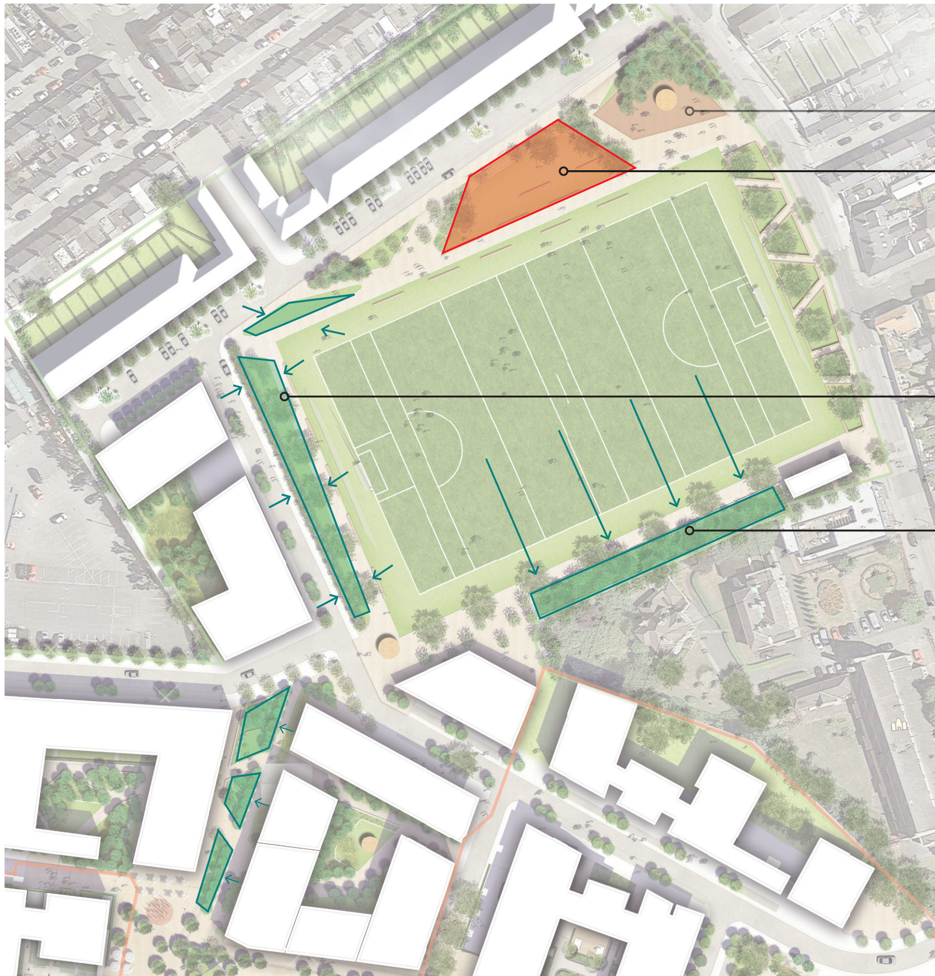
Fig. 4.29.5: Surface water management plan for GAA pitch
